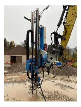
Attachable crawler track to 12 t excavator with the latest technology, high manoeuvrability (360° turn, 90° swivel and 600 mm shift) and very high torque. The drilling attachment is simply mounted to the excavator by means of a quick hitch and without tools. The control unit and the optional power supply are located in a package on the mount. The drill mast is radio remote controlled. The most important drilling parameters can be read on a digital display on the radio control.
