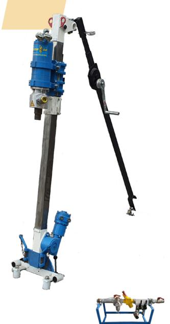
Lightweight, portable chain feed, fully pneumatic, ideal for all handy drilling operations; can be used with down-the-hole hammer as well as with drill hammer. Uncoiled for easy mounting on any type of scaffolding; suitable for wall work.
